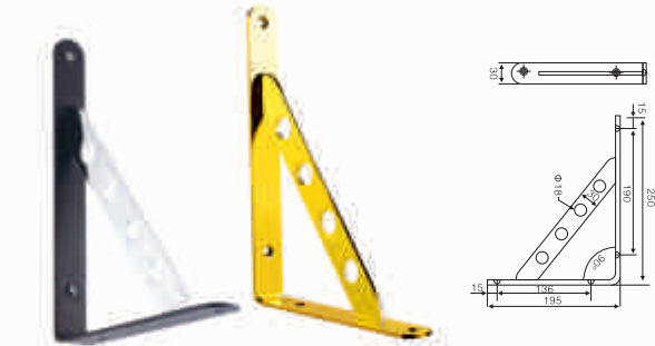
FJD-07-A01 MULTI-HOLE BRACKET COLOR: CHROME/NICKEL/ GOLD/ BLACK PLATED CARRYING CAPABILITY: 20KG
