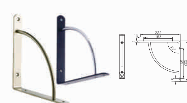
FJD-07-A04 SWING-LINE SHE SHELF BRACKETS COLOR: CHROME/NICKEL/ GOLD/ BLACK PLATED WEIGHT CAPACITY: 40KG
