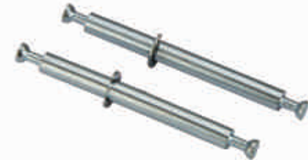
FJD-04-025 DOUBLE HEAD DOWEL DIA:6.8MM LENGTH:84-87MM FINISH: WHITE/YELLOW ZINC PLATED
