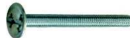
HANDLE SCREW HEAD: TRUSS HEAD/TRUSS WASHER HEAD SIZE: M4-0.7xL (L=12-100mm) M5-0.8xL (L=12-100mm) M6-1.0xL (L=12-160mm) M8-1.25xL (L=15-160mm) THREAD: METRIC FINISH: WHITE/YELLOW ZINC PLATED
